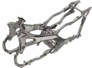
Robotically welded aluminum twin-spar frame with revised plate thicknesses in frame spars for optimized rigidity and flex characteristics. (Frame and swingarm are 4.4 pounds lighter.)
